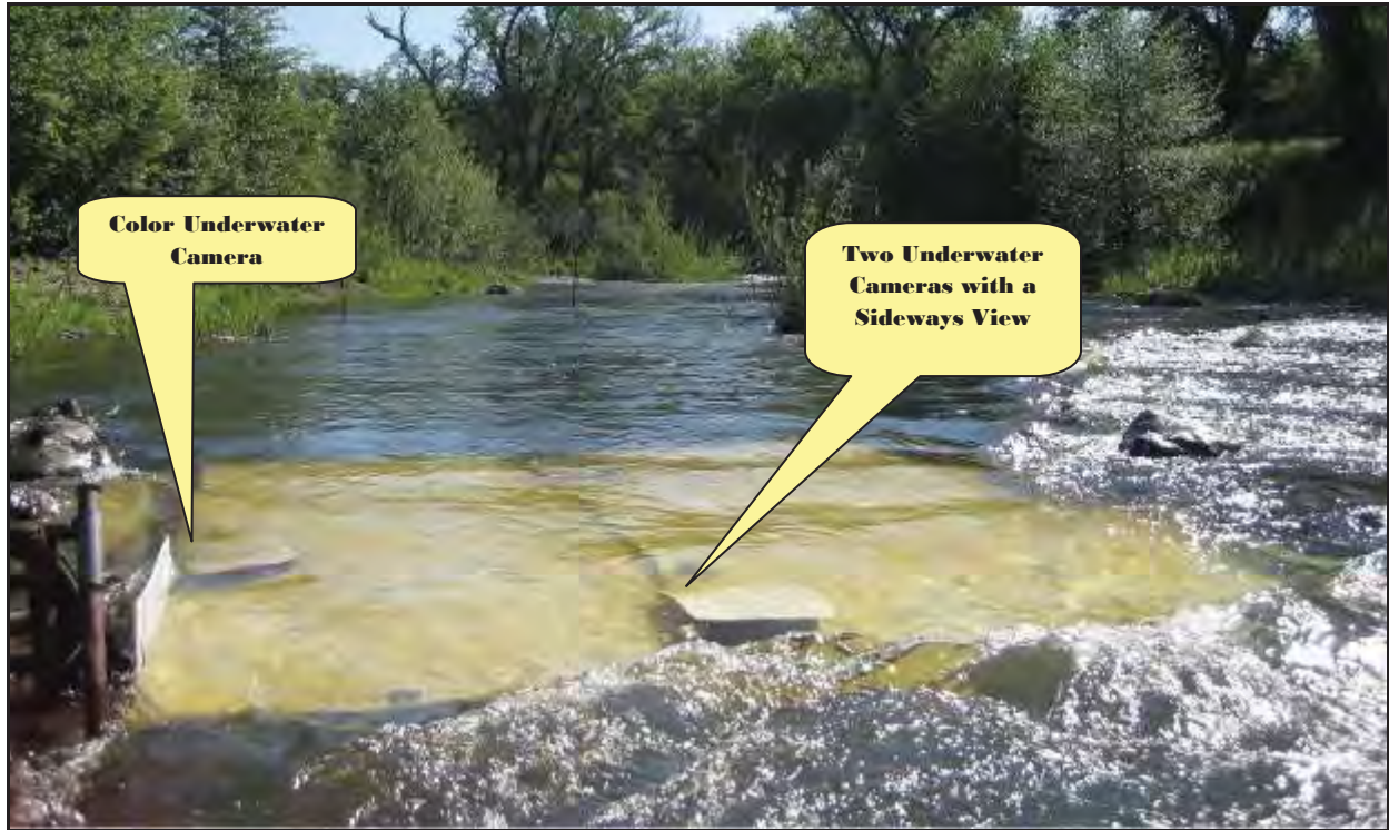
Figure 8. The underwater cameras were useful for monitoring up and downstream movement as well as species identification. The two middle cameras have a sideways view.
