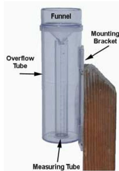
The rain gauge should be installed at a reasonable distance away from obstacles such as buildings and trees. For example, if a tree is 40ft. tall (taller than a two story house) the gauge should be placed at least 80ft. downwind from it. This will help avoid potential blockage of the rain gauge. It is not always possible to find a perfect location. **When in doubt, do your best.**
