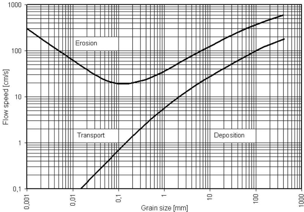
**Figure 5. Hjulstrom Curve**
