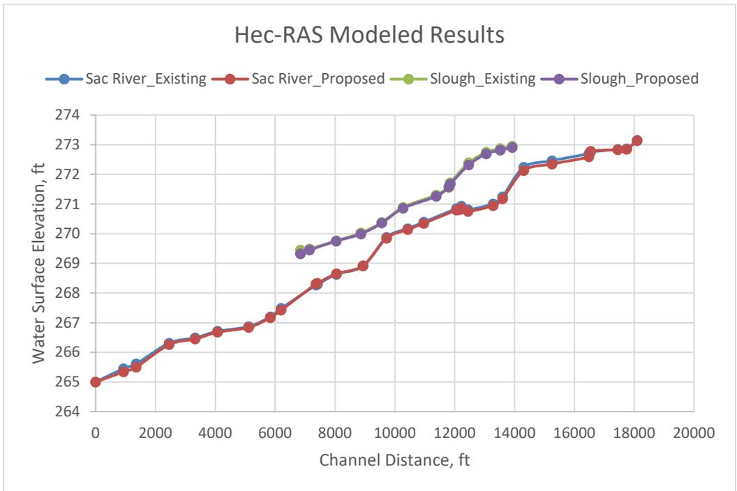
**Figure 3. Hec-RAS Proposed design modeled results**
